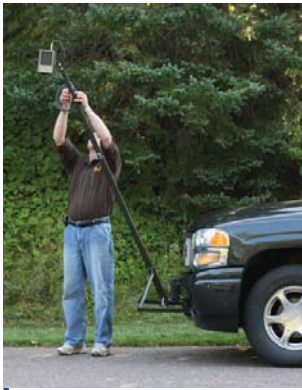
The BridgeGuard sensor unit is mounted on a mono pod on the front of a standard vehicle. Magnetic-mount GPS units are mounted to the vehicle's rooftop.
